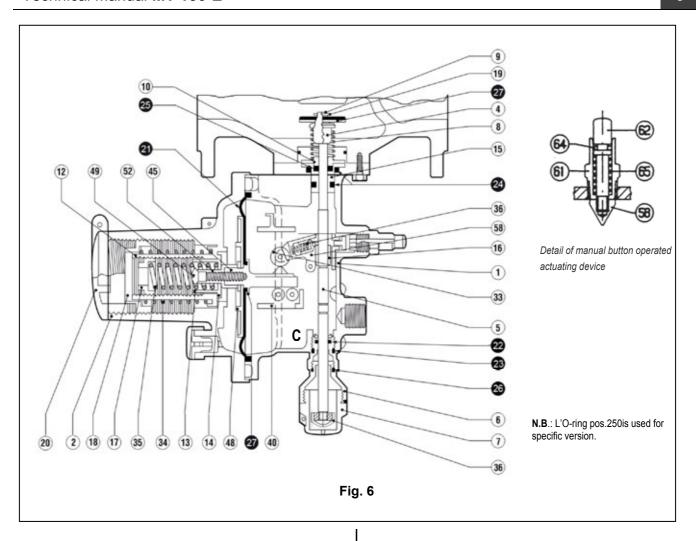
The slam-shut valve LA/.. consists essentially of an obturator (fig. 9) fitted on a stem, a releasing lever system, a control head and a manual resetting system. The pressure to control Pd, in chamber C of the control head, acts on the diaphragm 46 which is integral with the cam shaft 45.
