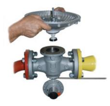
11) Separate the obturator group (200) from the head (300) by modifying the flowing-direction of the gas in order to get the shaft (203) getting out of the loading joint (312);
