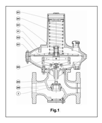
In fact, this solution allows the diaphragm protection disc 322 to rest on the upper stroke end V1 exceeding the load of the spring 331 and thus releasing the obturator from the load resulting from the sudden pressure increase.
