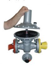
Completely unscrew the screw-nut (332) and take the spring out (331);
