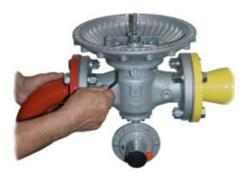
Separate the head (300) and the obturator group (200) from the regulator's body (1);
