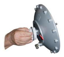
12) Tick off the obturator (204) from the stem (203) and separate gasket (205) from the obturator (204);
