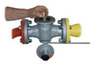
14) Unscrew then the screws (48) to dismantle the lower blind flange (10).
